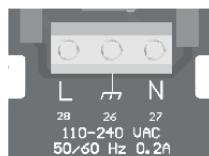
Connections alimentation principale 110–230 VAC
